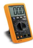
$\label{eq:special} \begin{tabular}{ll} (SPÉCIFICATIONS Tension CC: 200 mV-2/20/200/1000V. \\ Tension CA:: 2-20/200/700VCourant CC: 2/20/200 mA-20 \\ A. Courant CA: 2/200 mA- 20 A. Résistance: 200\Omega - 2/20/200 k\Omega - 2/20 M\Omega Capacité: 2/20/200 nF - 2/200 <math>\mu$ F.  $Température: -20^{\circ} + 1000^{\circ} C/ -4^{\circ} F & +2000^{\circ} FFréquence: 20kHz) \\ \end{tabular}$
