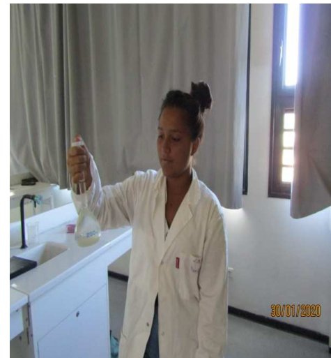
2. Dissolving the given mass of sugar in a 250 mL volumetric flask
