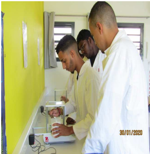
1. Weighing of a given mass of sucrose
